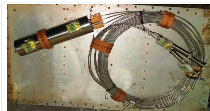
Figure 3: Detector arrangement for radiation ageing test.
