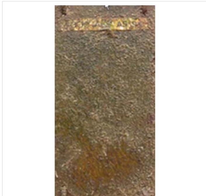
**Figure 7:** Exposure of the Re-Turn antifouling with 4 wt. %CuO (SeaNine™ 211) and anticorrosion paint in the Singapore sea waters.
