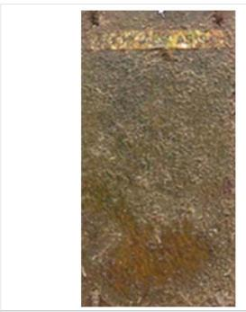
Figure 7: Exposure of the Re-Turn antifouling with 4 wt. %CuO (SeaNine™ 211) and anticorrosion paint in the Singapore sea waters.
