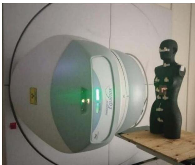
Figure 3: Irradiation of Alderson Rando phantom by <sup>60</sup>Co Teletherapy unit.
