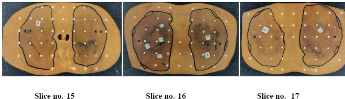
Figure 1: Inner view of lung targeted slice of Alderson rando phantom with TLDs.
