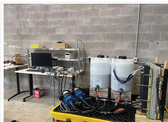
Figure 2: Shown is an assembled Ashlawn 3-cell medium-sized vanadium redox flow battery stack, with electrolyte tanks and pumps for the negative and positive battery half-cells, with a computer for monitoring the stack (on the bench in the left-hand background). Controls for adjusting pump speeds are shown on the bench with the computer. Spill berm (black lattice insulating structure inserted into the yellow tub) for fluid containment is shown below the tanks, pumps, and stack. (Taken from [10].)
