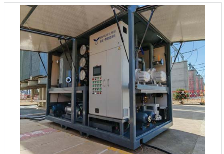
Figure 1: Transformer Oil Purifier [10].
